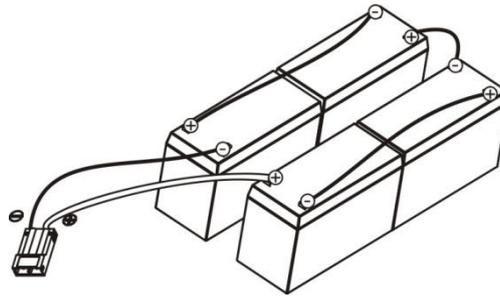
Step 3: Put assembled battery packs on one side of plastic shells.
