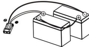
Step 3: Put assembled battery packs on one side of plastic shells and insert one more defect battery on the space.
