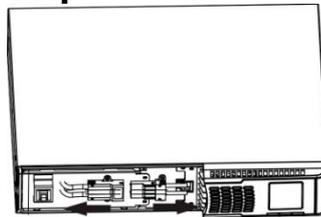
Disconnect battery wires.
